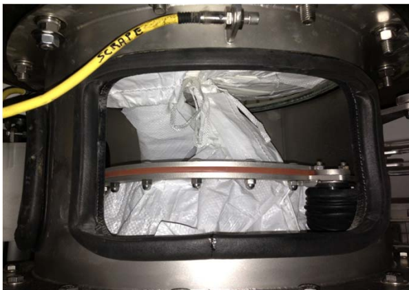
3. Pull both exterior handles to seal the spout
