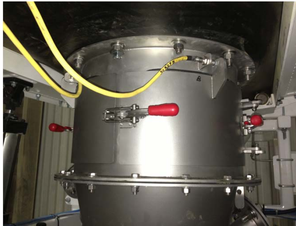
1. Unlatch 3x toggle clamps to open both access doors
