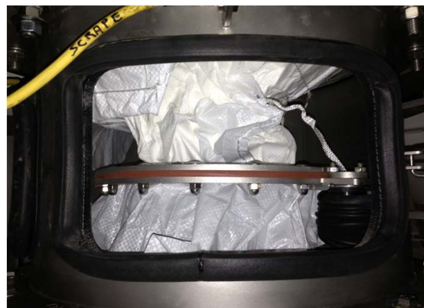
5. Untie bulk bag's discharge spout knot to let product flow freely
