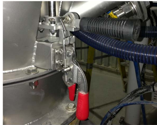
4. Lock sealing device with both toggle clamps
